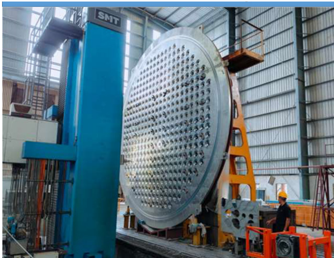
End Shield Assembly for 700 MWe fleet mode reactor on the new CNC Skoda Horizontal Boring Machine
