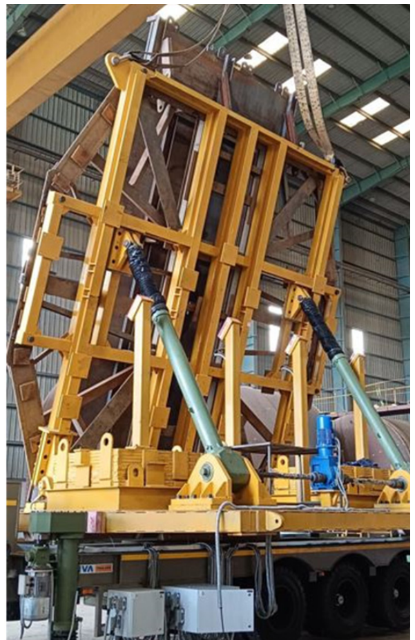
First of its kind design and Development of fixture for testing of ship based antenna system
